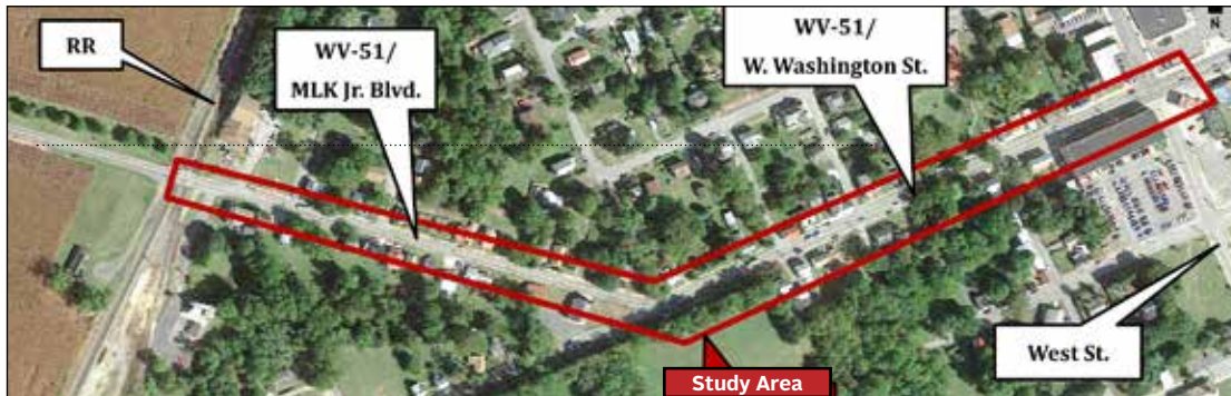
(Above, left) The WV-51 feasibility study is looking at vehicular, pedestrian, and bicycle safety and mobility improvements in this vicinity, and evaluating the options of a roundabout, traffic signal, or other traffic control alternative at the intersection. Along with the traffic control and calming, the study is looking at accessible sidewalks and curb ramps, a bicycle lane, pedestrian crossings (including mid-block at Evitts Run park), street parking, utility relocation, and stormwater management along the study corridor.
