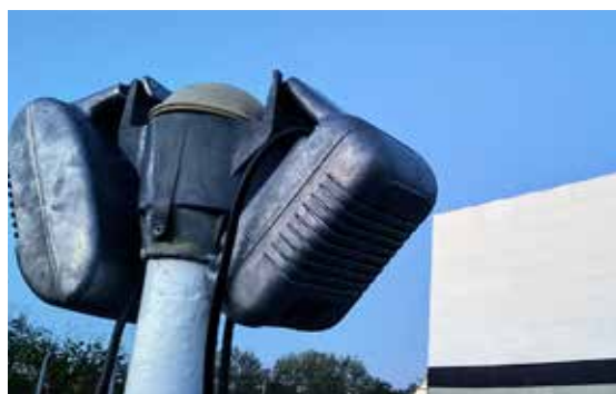
In addition to broadcasting sound via FM to your vehicle's stereo system, the theater still operates the 1950s vintage pole speakers (with mono-channel sound).
