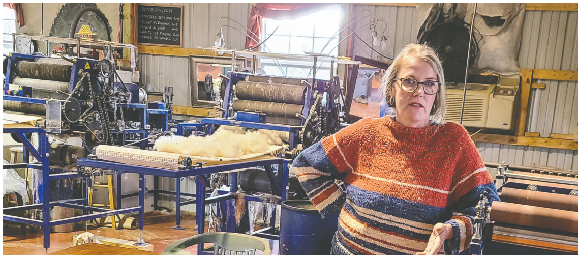
Bridget Brown explains how a fleece is processed in the fiber mill. After the raw fleece is washed it (1) goes through a picker to loosen the fibers, then (2) it then runs through a carding machine (behind Brown) which creates a loose fluffy "roving" and then (3) through the draw frame which tightens up the roving. The final step (4) is a trip through the spinning machine (image above, right).
