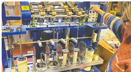
(above) The spinning machine can spin four single threads, which can in turn be combined to create 2, 3, or 4 ply yarn (with the option to mix wool from different animals to create unique blends).
