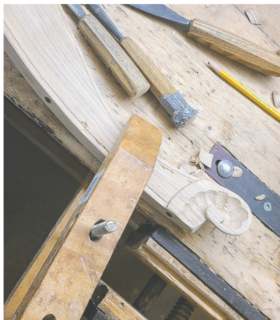
The workshop is a small-scale factory, even if it looks a bit rustic. The manufacturing process includes lots of carving (above, left) handwork (above, upper right). A typical Windsor chair is constructed with four types of wood for a balance of comfort and functionality. Once complete (above, right) chairs and tables can be hand-painted in any color and finish.
